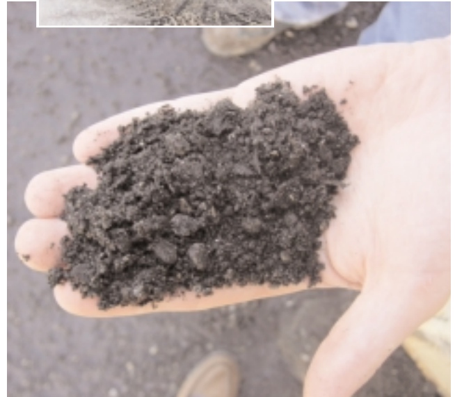
Shingles are finely-ground before entering the asphalt plant
